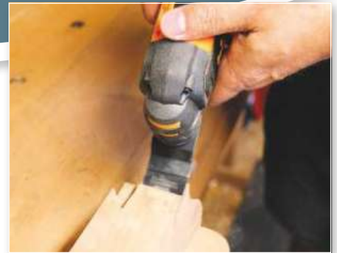
▲ There's plenty of power for such a small unit – this 32mm cut in beech was easy
